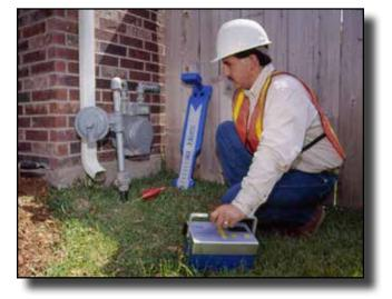
A unique feature of the All Pro is "continuous depth" readings. No need to press a button for your depth, a depth reading is continually displayed on the receiver as you near the target conductor.
