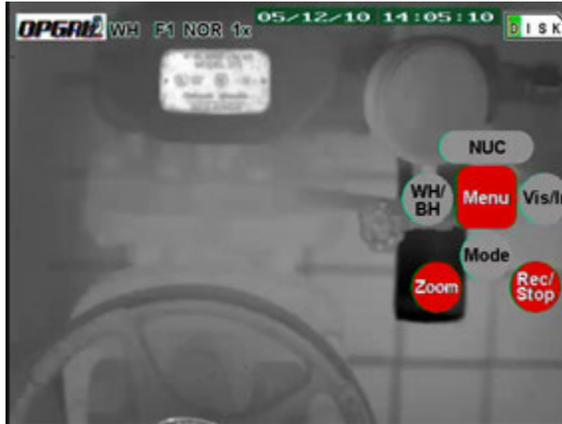
Figure 5: Keypad mapping on LCD
