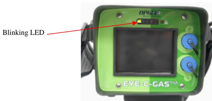
**Figure 19: Logo and LED blinking during cool down**
